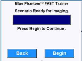
Select BEGIN from on the touch panel. Once the user has selected BEGIN from the touch panel, a timer keeps track of the time from selection until the user enters the detected effusion state.
